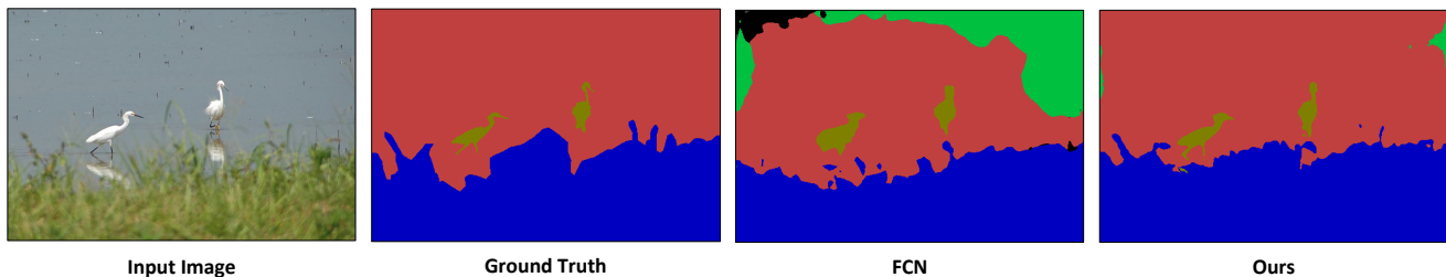
Figure 4. Segmentation results on PASCAL-Context 59-class. Our approach uses an MLP to integrate information from both lower ( e.g. l_2 ) and higher ( e.g. conv-7 ) layers, which allows us to better capture both global structure (object/scene layout) and fine details (small objects) compared to FCN-8s .
