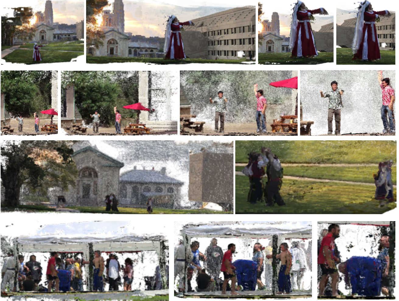
Figure 23. Dense 3D reconstruction from sparse views: We show dense 3D point clouds computed using our approach for a specific time instant for four unconstrained multi-view sequences [3]. A user can easily explore the region by navigating the point clouds. We show random views of the point clouds.
