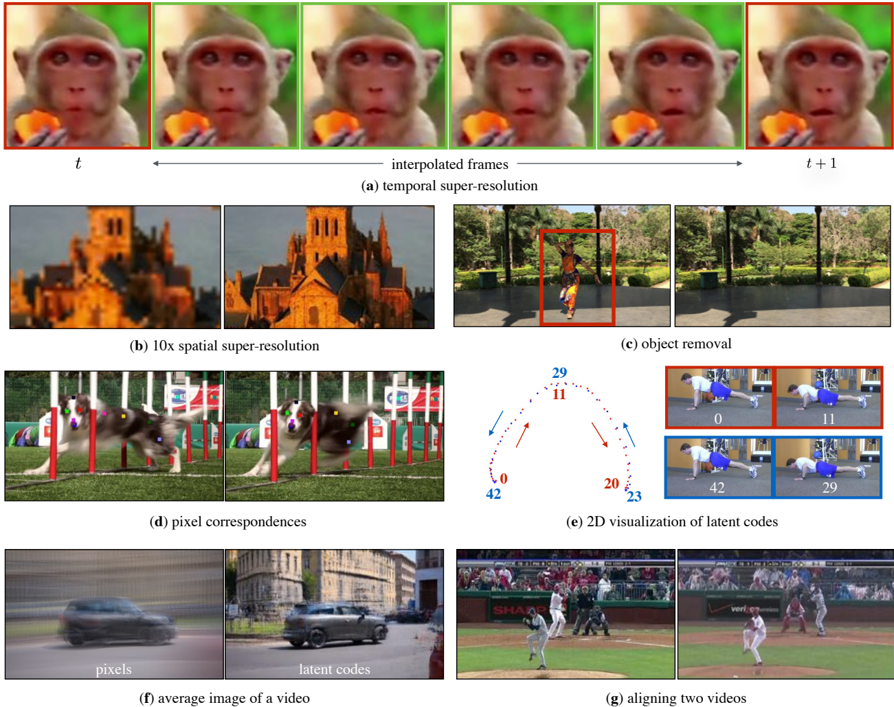
Figure 30. We demonstrate a remarkable number of video processing tasks enabled by a simple video-specific representation: an image autoencoder trained on frames from a target video. (a) By interpolating latent codes of adjacent frames (and decoding them), one can perform temporal super-resolution . (b) By linearly upsampling low-res 96 \times 96 image frames to 1024 \times 1024 blurry inputs and passing them through the autoencoder, we can project such blurry inputs into the high-res-video-specific manifold, resulting in high quality 10X super-resolution , even on subsequent video frames not used for training. (c) Manifold projection can also be used to remove objects marked with a bounding box. (d) Hypercolumn features of the autoencoder can be used to establish per-pixel correspondences across frames of a video via feature matching. (e) Multidimensional scaling of latent codes (via 2D Principal Component Analysis) allows for “at-a-glance” interactive video exploration; one can summarize visual modes and discover repeated frames that look similar but are temporally distant. (f) We can summarize videos by decoding the average latent codes (of all the frames in a video), which compares favorably to a naive per-pixel average image. (g) Manifold projection allow us to align two semantically similar videos and retarget from one to another (here, two baseball games).
