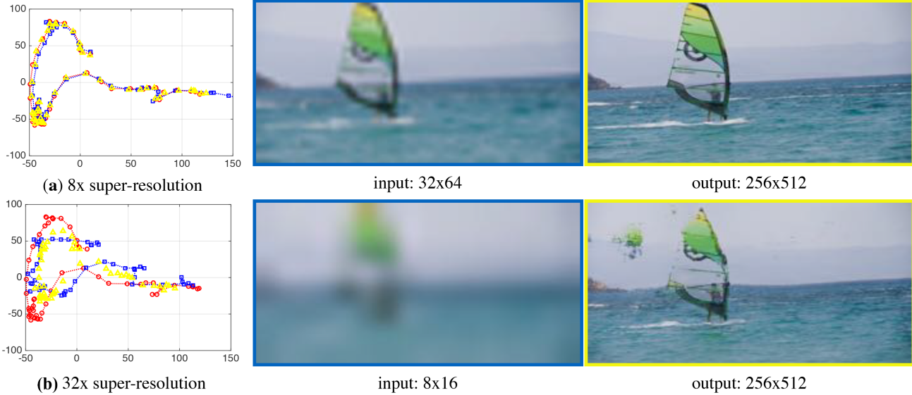
Figure 2. Manifold Projection with autoencoders: We train a video-specific autoencoder on 55 high-res 256 \times 512 frames. We visualize the latent codes for the original frames using the red points on the left side. At test time, we input low-res versions of held-out frames of varying resolution. We visualize the latent codes for the low-res input using the blue points. We also visualize the latent codes for the output image using the yellow points. We observe that red points, blue points, and yellow points for (a) 8X super-resolution. We observe perfect reconstruction for this input. The results, however, degrade as we further reduce the resolution of images, as seen in (b) 32X super-resolution.
