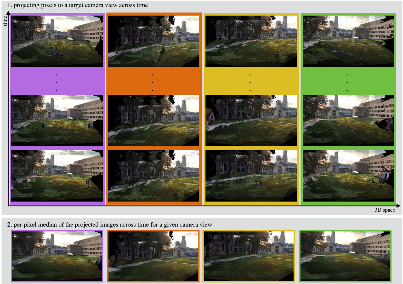
Figure 5. Static Background Estimation: (1) We use the pixels corresponding to the farthest 3D points (from the per-pixel cost volume of depth) to generate an image for a target camera pose and time instant. This enables us to get the farther components of the scene that are often stationary. However, this information is noisy. We, therefore compute the images for a given camera pose across all time. (2) A per-pixel median of the images over a large temporal window for a target camera pose results in a smooth stationary background.
