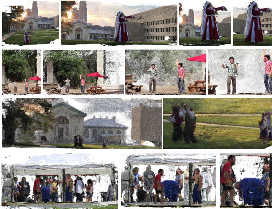
Fig. 22. Dense 3D reconstruction from sparse views: We show dense 3D point clouds computed using our approach for a specific time instant for four unconstrained multi-view sequences [3]. A user can easily explore the region by navigating the point clouds. We show random views of the point clouds.
